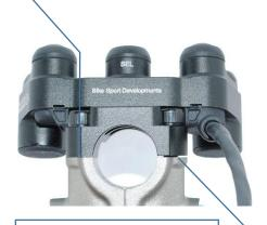
1.0mm of gap – Used for tightening the clamp.21.5 > 22.2mm dia bar
